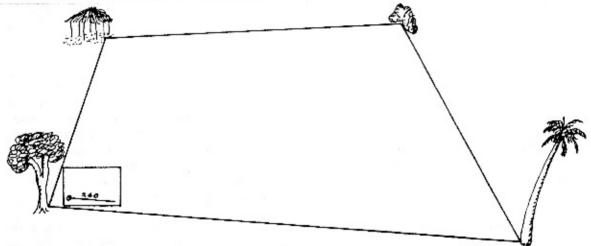
The board is then taken to the second point, laid on the ground, and oriented by sighting along the line drawn on the paper with the help of the ruler so that the line is lined up pointing back to the first point. Holding the board carefull so that it does not move, the ruler is then placed so that it crosses through the second point and is sighted at the third point. A line is then drawn, paced and measured as before, and the third point is marked and labeled.
