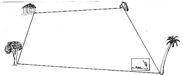
At each corner or point along the boundary to be mapped, the board is placed on the ground and the same procedure is followed. If there is some error in closing the boundary when returning to the first point, it can usually be adjusted in redrawing the map.
