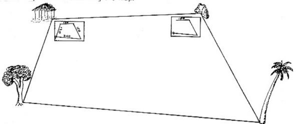
If the area to be mapped is very large, it is best to subdivide it into smaller sections, map them separately, and then join the pieces of the map together. Other features to be added to the map that are not on the boundary lines can be added by sighting to them and pacing off the distance. If they are far off the line, it is best to sight and pace from two points on the line, forming a triangle, at the point of which the feature is marked.
