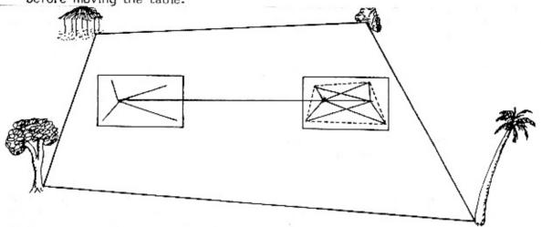
Once the positions of the major reference points have been located on the map, it should not be too difficult to draw in boundaries, important landmarks, and detailed features, and to add appropriate labels to make the final map. The sight lines used to prepare the map can be erased when they are no longer needed, or the map can be recopied in its final form.
